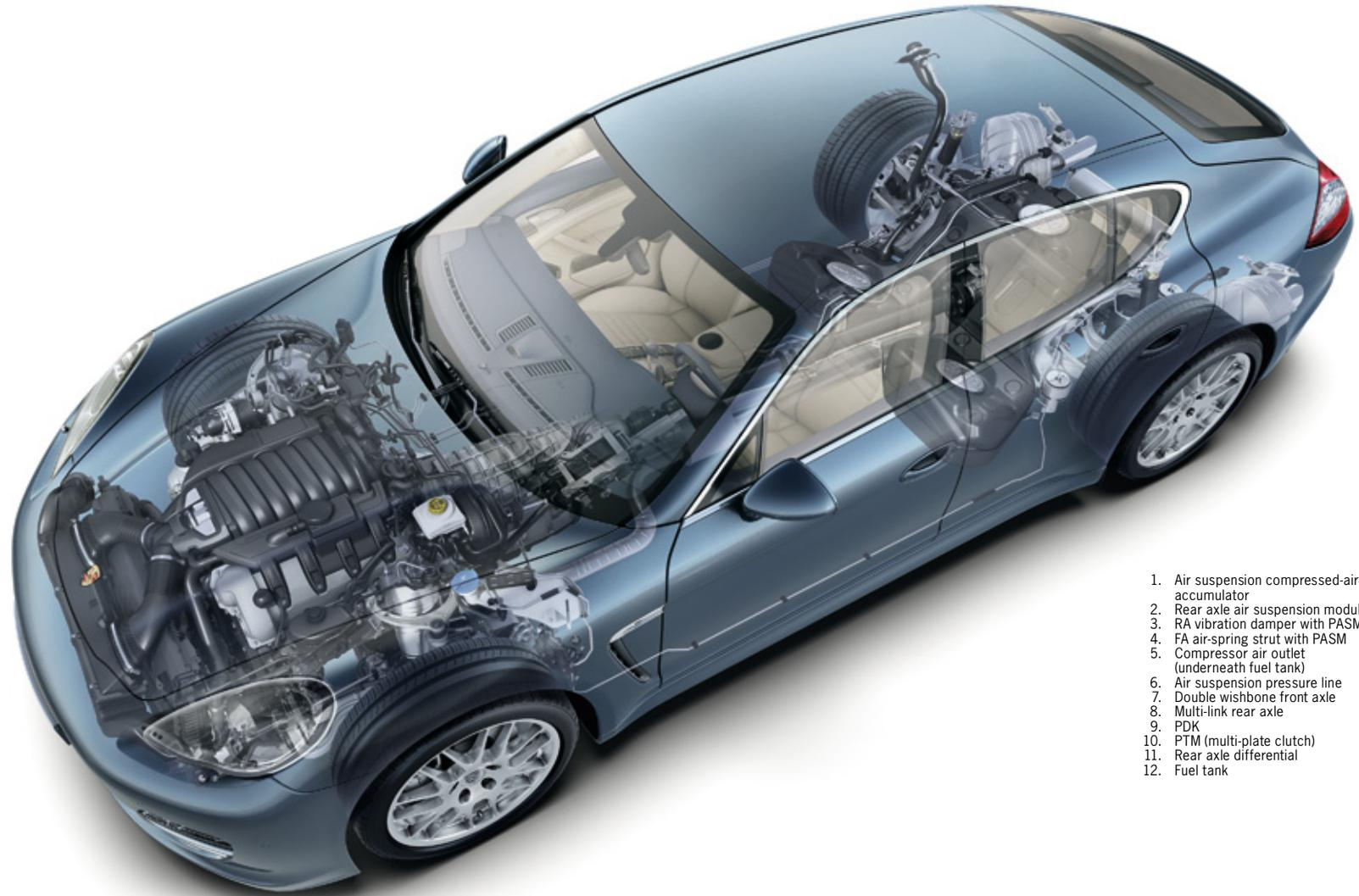
1. Air suspension compressed-air accumulator
