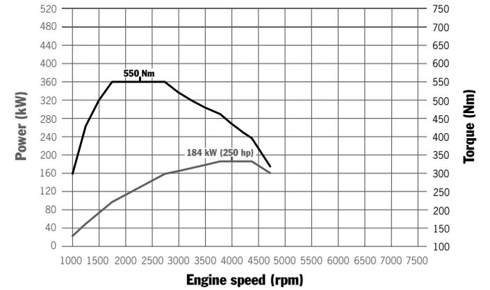
Panamera Diesel: 184 kW (250 hp) at 3,800–4,400 rpm, 550 Nm between 1,750 and 2,750 rpm
