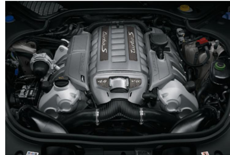
The V8 twin-turbo engine in the Panamera Turbo S
