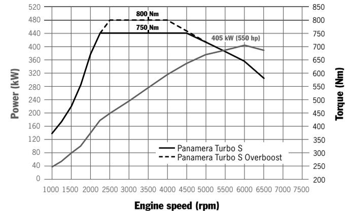
Panamera Turbo S: 405 kW (550 hp) at 6,000 rpm, 750 Nm (800 Nm with overboost) between 2,250 and 4,500 rpm
