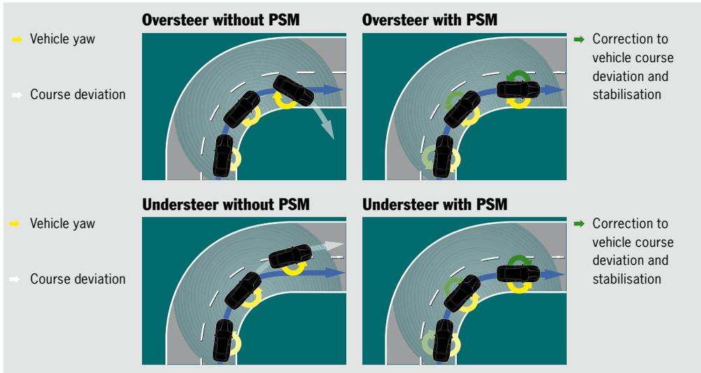
For a more dynamic experience, you always have the option to deactivate PSM. It is automatically reactivated, for your safety, only if you brake harder and either of the front wheels (in SPORT PLUS mode, both of the front wheels) requires ABS assistance.
