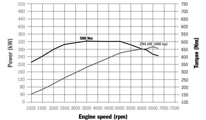
Panamera S and 4S: 294 kW (400 hp) at 6,500 rpm, 500 Nm between 3,500 and 5,000 rpm
