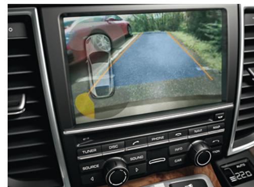
Image from reversing camera in PCM
