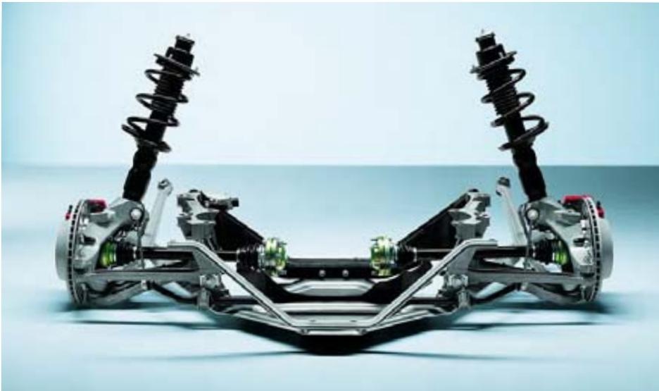
MacPherson rear axle with suspension struts and transverse links (Boxster S)
