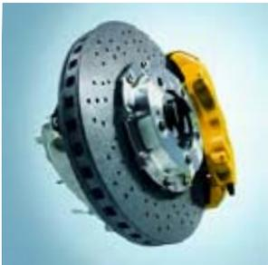
To maximize cooling in extreme track conditions, the latest evolution of PCCB has a modified system of internal vents, with twice the number of cooling channels. This vent geometry facilitates airflow through the disc and, with double the number of channels, there are more internal walls for greater structural stability.
