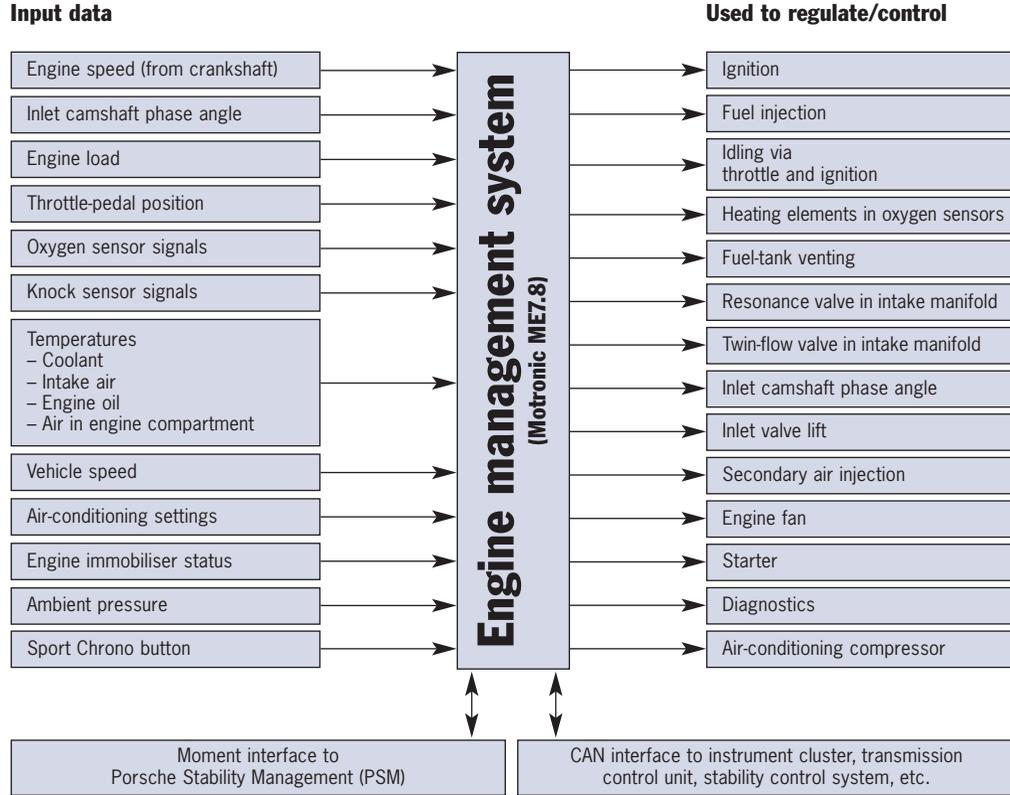
**Engine management system with electronic throttle.**
