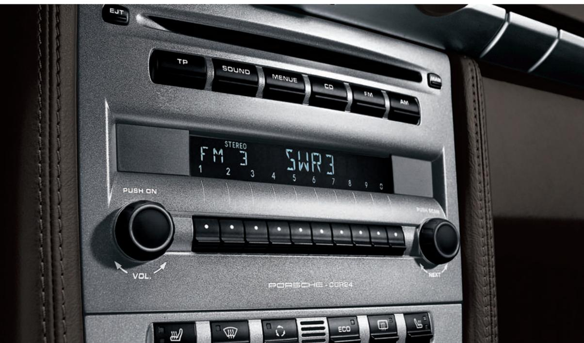
The Boxster audio system offers exceptional sound reproduction. Two high-range speakers on the dashboard, two low-range speakers in the doors and two 25-watt amps give audiophiles a superior starting point for complementing the aural delights of the flat-six engine's exhaust note at speed.
