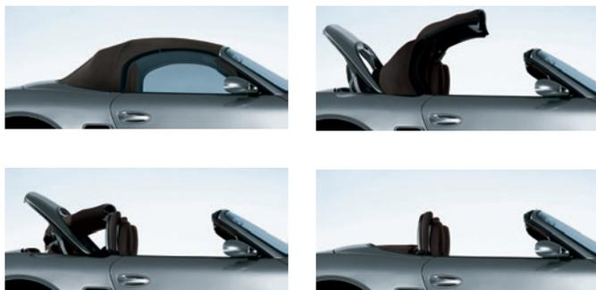
A zig-zag folding action protects the interior roof lining when the top is stowed away. The interior is lined with a stylish and practical sound-insulating fabric that reduces interior noise.
