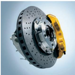
To maximize cooling in extreme track conditions, the last evolution of PCCB has a modified system of internal vents, with twice the number of cooling channels. This vent geometry facilitates airflow through the disc and, with double the number of channels, there are more internal walls for greater structural stability.
