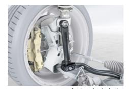
Coupling rod made of carbo
