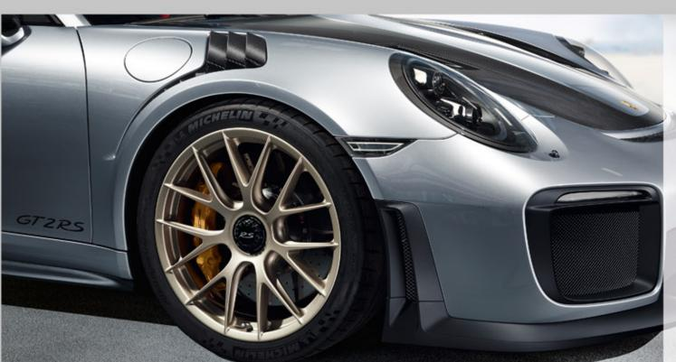
From lightweight plastic to lightweight metal. The magnesium wheels painted in satin White Gold Metallic make the new 911 GT2 RS fitted with the Weissach package approximately 11.5 kg lighter and also enhance its visual appearance. A double victory, so to speak.
