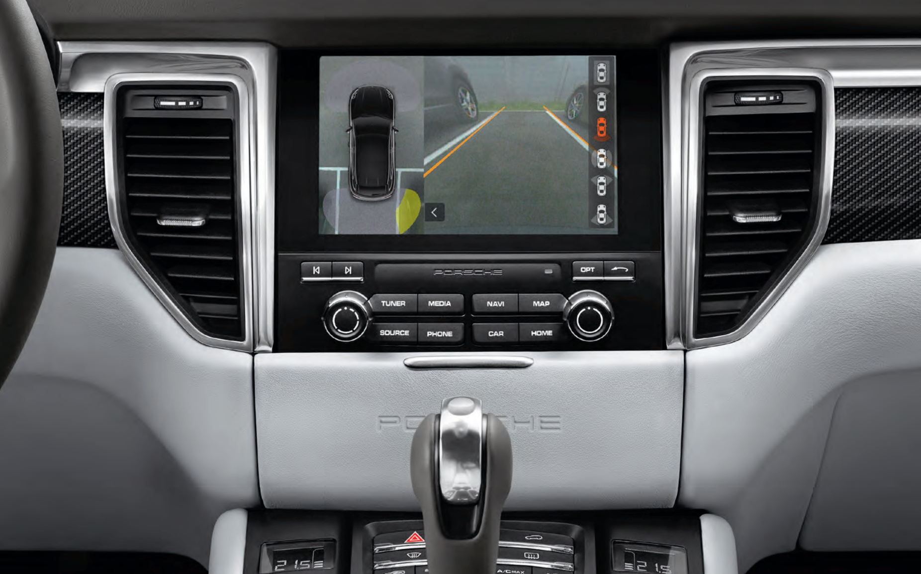
ParkAssist including reversing camera and Surround View
