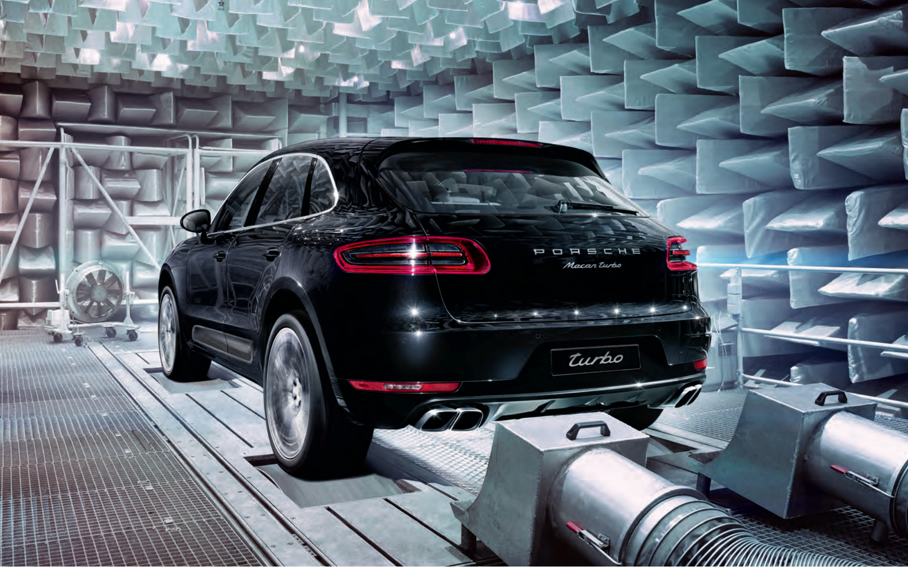
Acoustic test chamber in Porsche Development Center, Weissach
