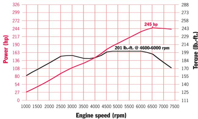
Cayman: 201 lb.-ft. between 4600 and 6000 rpm, 245 horsepower at 6500 rpm
