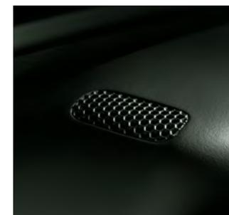
AudioPilot system microphone mounted left of the steering column to monitor interior noise level
