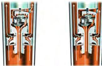
Left: Compression in Normal mode—bypass valve open
