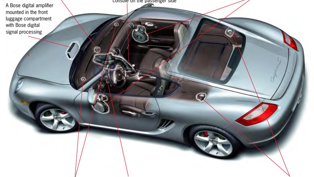
A Bose digital amplifier mounted in the front luggage compartment with Bose digital signal processing
