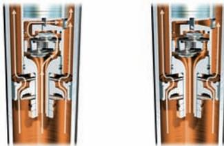
Left: Compression in Normal mode—bypass valve open
