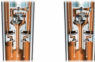
Left: Rebound in Normal mode—bypass valve open
