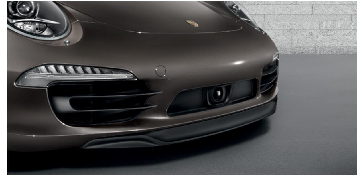
Radar sensor of adaptive cruise control
