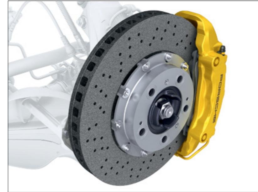
The use of six-piston aluminium monobloc brake calipers on the front axle and four-piston units at the rear – all finished in yellow – ensures extremely high brake forces which, crucially, are exceptionally consistent.
