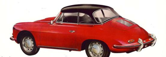
Wind wings in front and rear Wind wings in front and rear Glare-proof rear view mirror Laminated safety glass windshield FM suppressed windshield wipor motor Ventilated rear window (except Cabriolet) Cabriolet rear window with zip fastener
