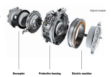
On the parallel full hybrid system, the electric machine is integrated directly into the drivetrain. The hybrid module is situated between the transmission and the combustion engine. The engine is engaged and disengaged using a specially designed decoupler.
