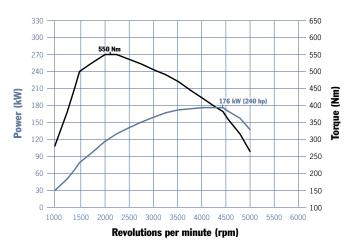
Cayenne Diesel: 550 Nm between 2,000 and 2,250 rpm, 176 kW (240 hp) between 4,000 and 4,400 rpm
