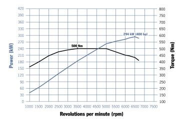
Cayenne S: 500 Nm at 3,500 rpm, 294 kW (400 hp) at 6,500 rpm
