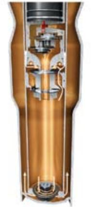
Compression in 'Normal' mode – working piston and bypass, sporty-hard tuning
