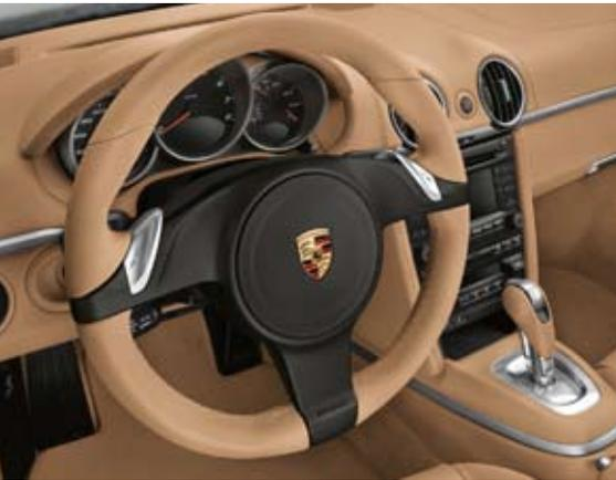
Three-spoke sports steering wheel with gearshift switches
