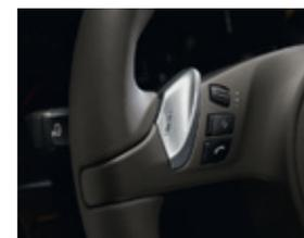
PDK gearshift switches on multifunction steering wheel
