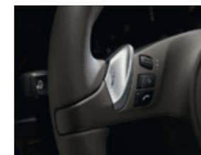
PDK gearshift switches on multifunction steering wheel
