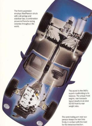
The 968's five-spoke turbo design wheels are made of cast aluminum to reduce unsprung weight for enhanced handling agility. The open design helps the brakes cool under hard or
