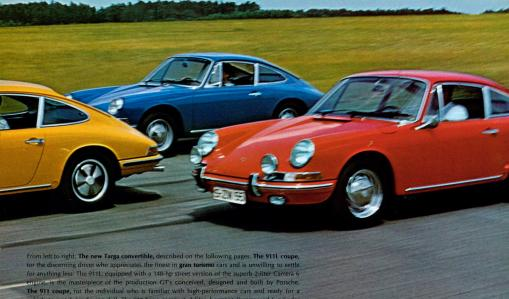
vehicle to match his driving skill. The 911 has a compact, 2-liter, horizontally opposed 6-cylinder engine with overhead camshafts, delivering 148-hp. The 912 coupe, an excellent choice for the driver making his first venture into the high-performance field. The 912 is powered by Porsche's famous 102-hp air-cooled 4-cylinder engine.
