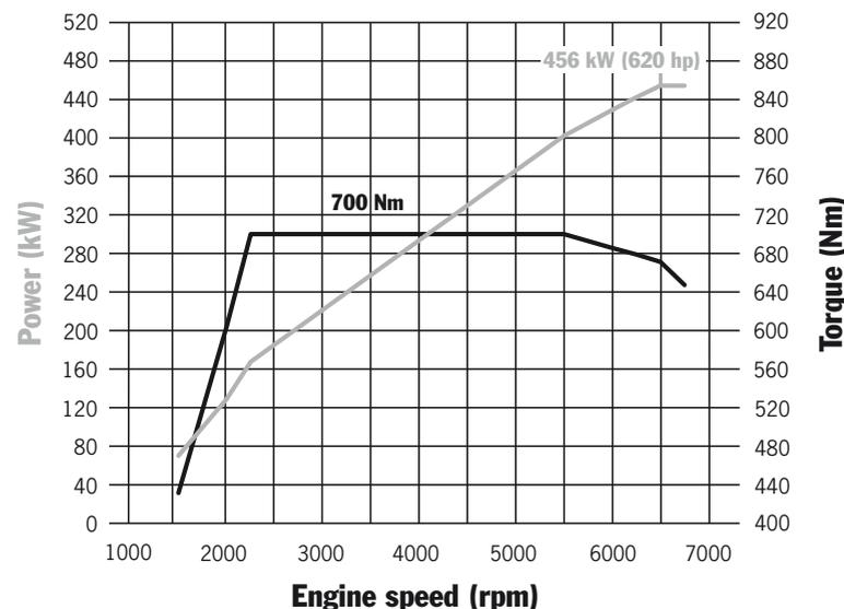
911 GT2 RS: 700 Nm at 2,250 rpm, 456 kW (620 hp) at 6,500 rpm
