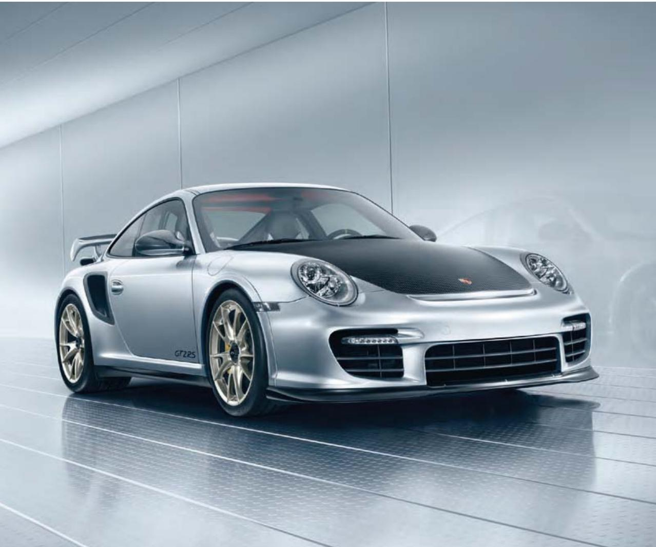
Front lid and side air intakes for the charge air cooler in carbon
