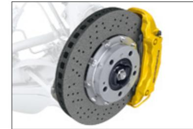
PCCB enables shorter braking distances in even the toughest road and race conditions. Excellent fade resistance ensures greater balance when slowing from racetrack speeds.
